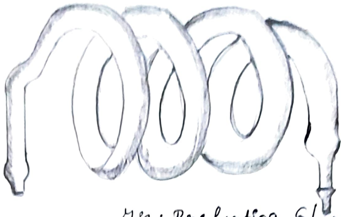
Fig: Preheating glass coil
